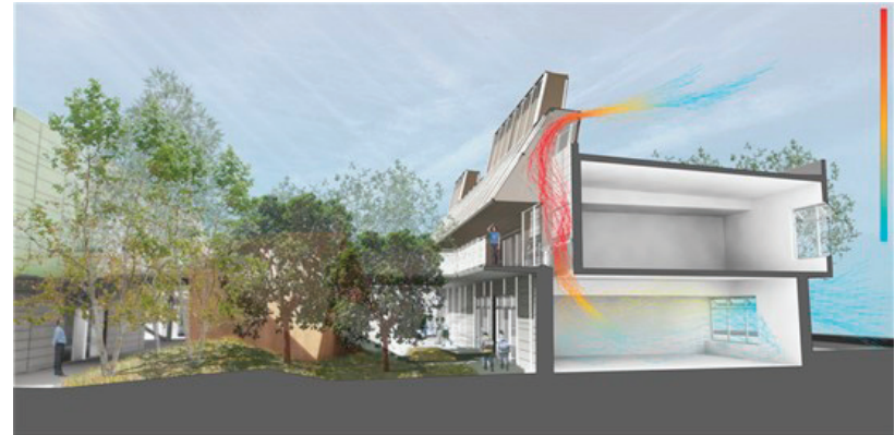
Thermal stack used to ventilate a classroom in Los Angeles. Image courtesy of Daly Genik Architects.
