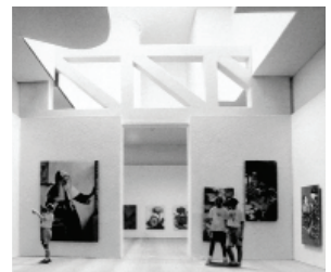
Physical model used to predict daylight quality
