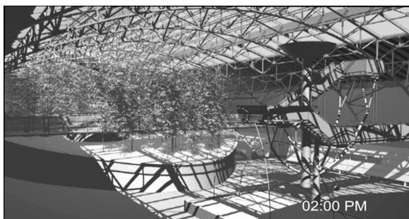
Figure 3: Sun and shade simulation. Perspective view looking northeast at 2:00 pm on the equinox.
