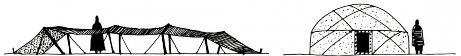
Portable tents of sticks and felt. Left: Arab tent. Right: Mongol Yurt.
